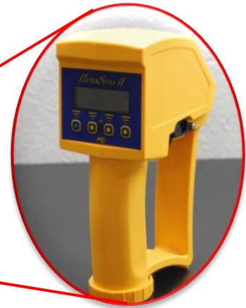
Used for internal room monitoring (0-2,000 ppm)
